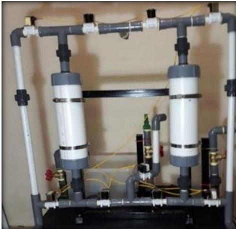
Gambar 17. Rangkaian unit *iron removal filter* (IRF).
