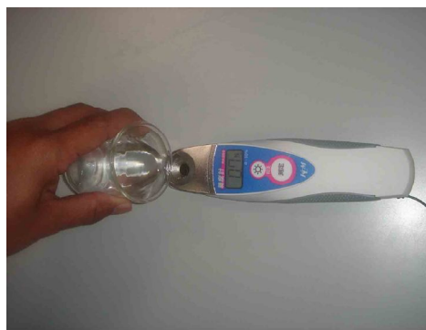
Figure 4. Measurement of concentration of sucrose solution using portable Brix meter.
