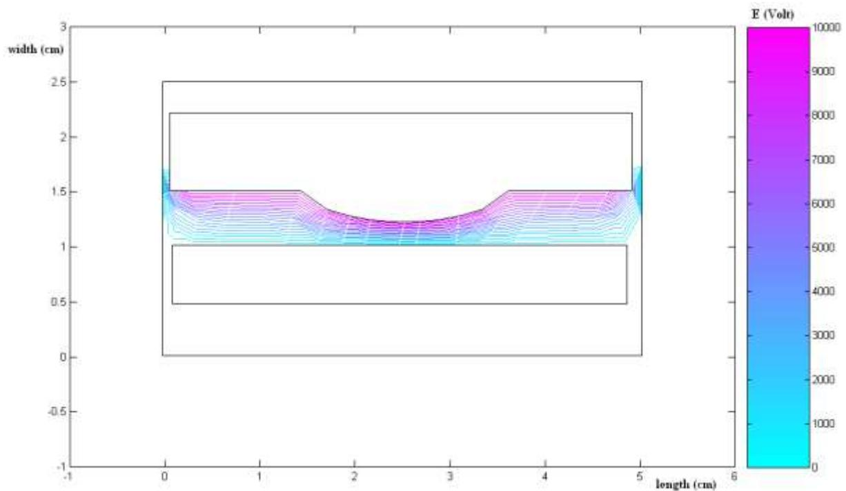
**Figure 2.** Electric field at a bulge type copper electrode.
