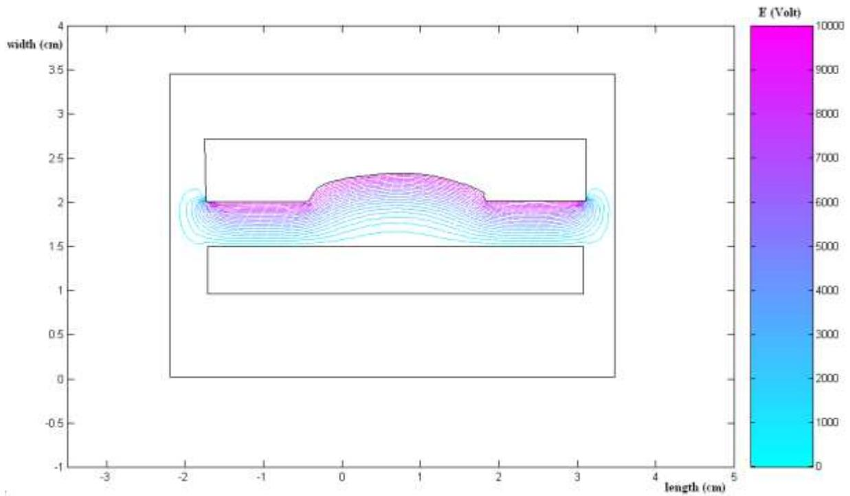
**Figure 1.** Electric field at a hole type copper electrode.
