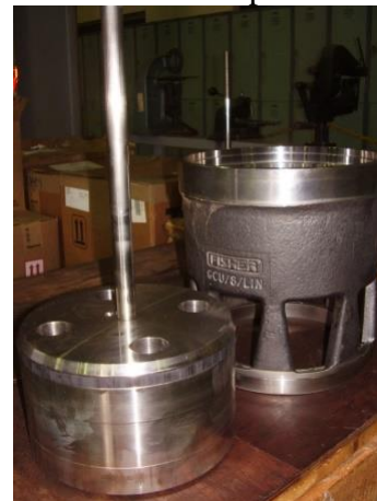
Gambar 11. Cage Valve Jenis Equal Percentage .
