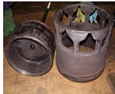
Gambar 10. Cage Valve Jenis Linier .
