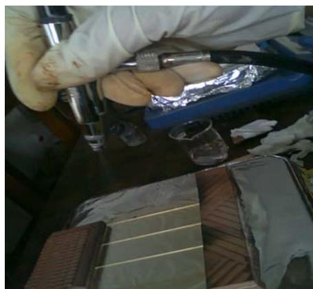
Gambar 1. Teknik *thermal spray coating*
