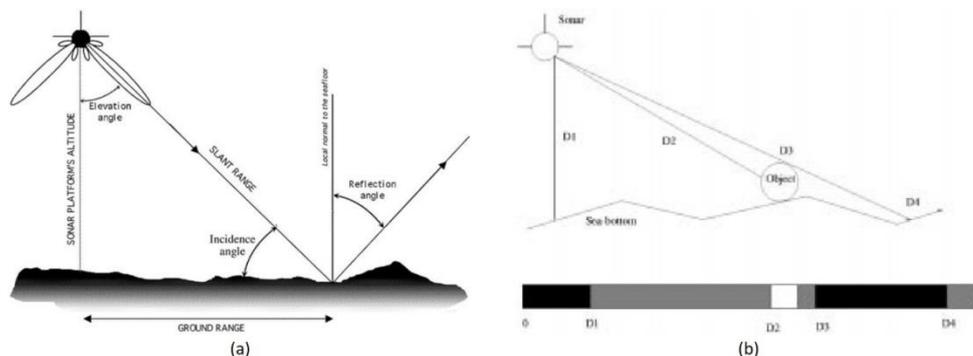
Figure 2.(a) Side-scan sonar signal propagation (Blondel, 2009), (b) Image construction (Daniel *et al.*, 1998)
