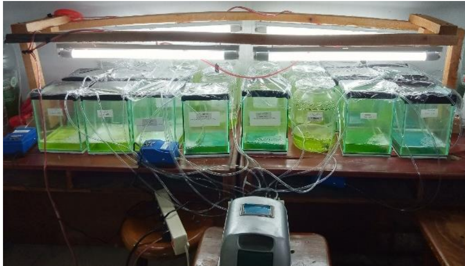
Figure 2. Lab Scale Phycoremediation with Chlorella vulgaris
