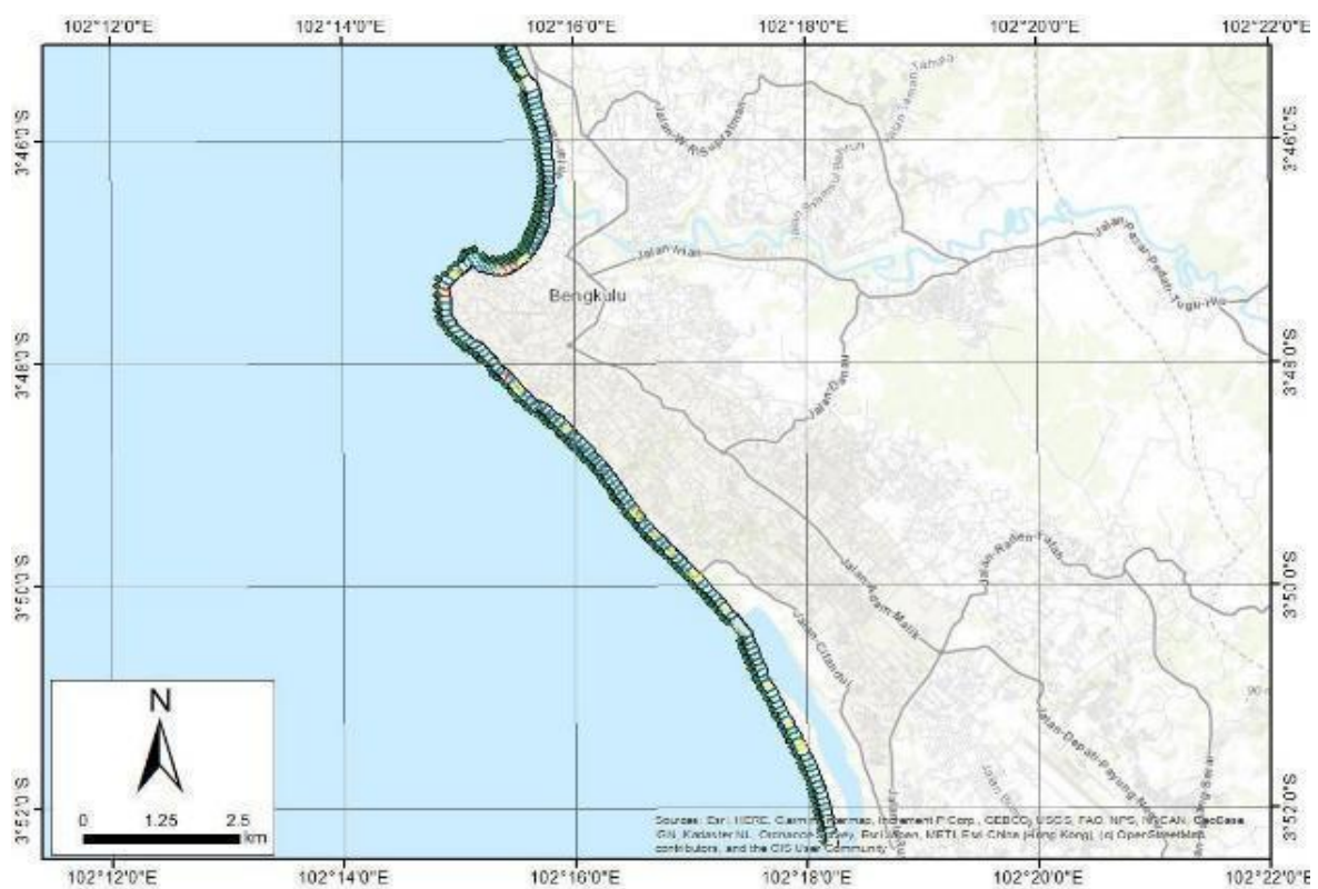
Figure 6. Annual shoreline change in Bengkulu to denote accretion (green lines), abrasion (red lines), and stable (yellow lines) from August 2020 to 2025.
