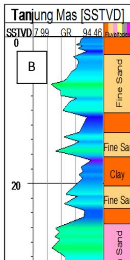
**Fig. 4.** Wenner inverse model of line Tg Mas in Tanjung Mas well station (A), Lithology of Tanjung Mas subsurface derived from interpretation of gamma ray data (B). (gamma ray data derived from Abdul Rashid 1989)
