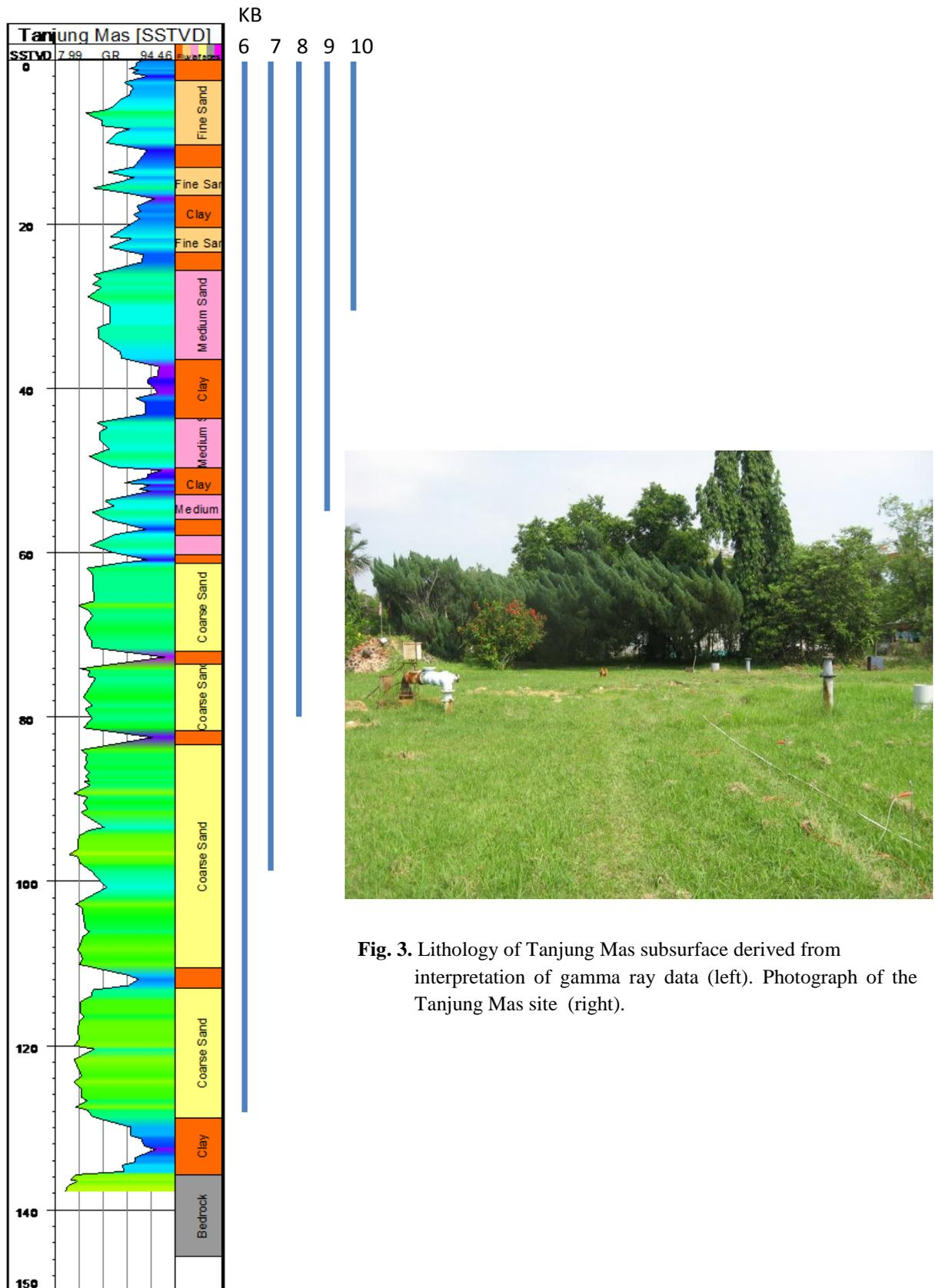
**Fig. 3.** Lithology of Tanjung Mas subsurface derived from interpretation of gamma ray data (left). Photograph of the Tanjung Mas site (right).
