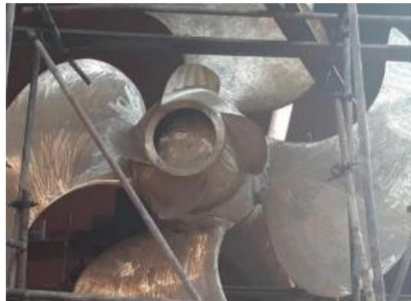
Gambar 1. *Propeller Hub Caps Fin*
