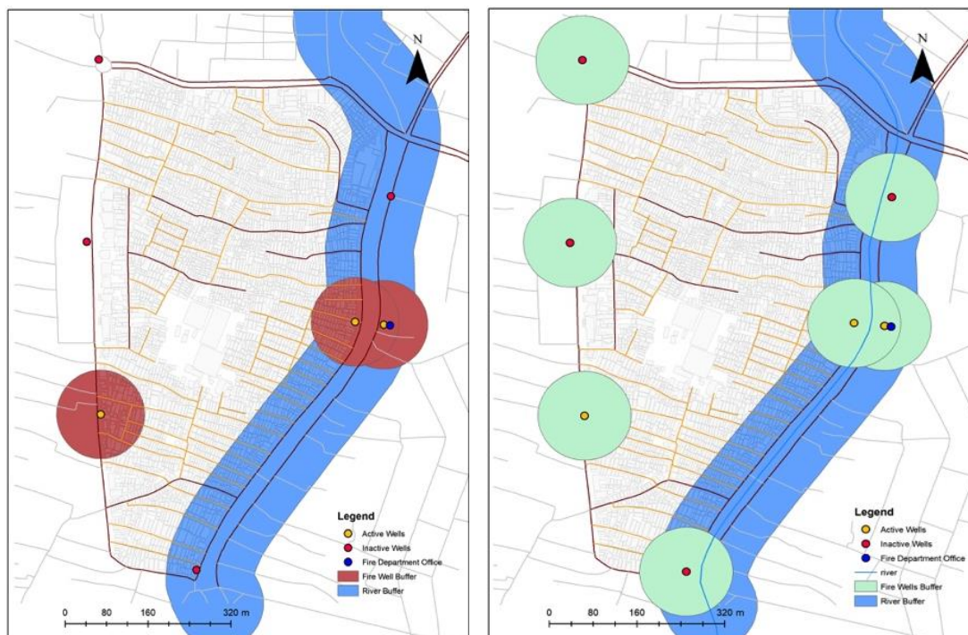
Figure 2. Comparison of fire resources buffer before and after reactivation of inactive fire wells
