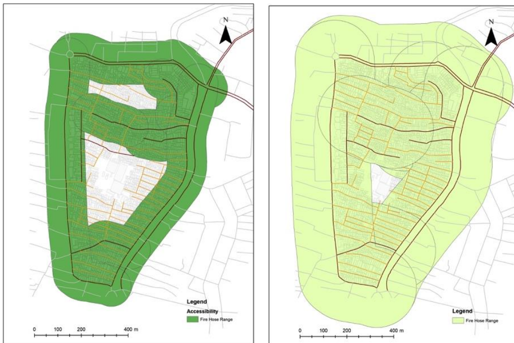
Figure 7. Comparison of fire hose range buffer before and after the installation of the fire hose adapter
