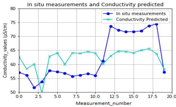
**Figure 4.** In-situ Measurements and Conductivity Predicted using the Adagrad Optimization
