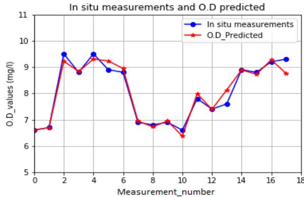
**Figure 10.** In-situ Measurements and Dissolved Oxygen Concentration Predicted using the Adam Optimization
