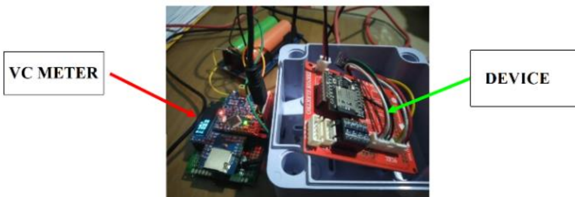
Figure 9. Power measurement using voltage-current meter
