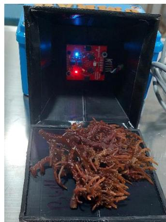
Figure 5. Seaweed (*K. alvarezii*) sample placed in the black box containing the AS7265x sensor for spectral measurement.
