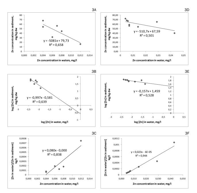
Figure 3. Different adsorption model for Zn in north stream (N) and south stream (S): 3A) N Partition model; 3B) N Freundlich model; 3C) N Langmuir model; 3D) S Partition model; 3E) S Freundlich model and 3F) S Langmuir model.
