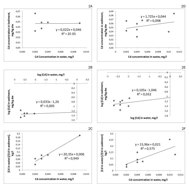
Figure 2. Different adsorption model for Cd in north stream (N) and south stream (S): 2A) N Partition model; 2B) N Freundlich model; 2C) N Langmuir model; 2D) S Partition model; 2E) S Freundlich model and 2F) S Langmuir model.
