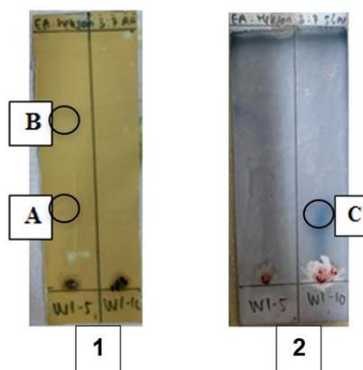
**Figure 7.** Phytochemical Screening of Separated Fractions with TLC: (1) Test for the presence of phenolics by spraying with FeCl<sub>3</sub> ; (2) Test for the presence of terpenoids by spraying with vanillin-sulfate; (A) Spot A; (B) Spot B; (C) Spot C
