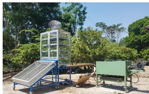
Fig 2. Complete view of hybrid solar dryer
