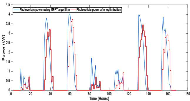
**Fig. 4.** Photovoltaic power reduction employing MILP optimization algorithm.
