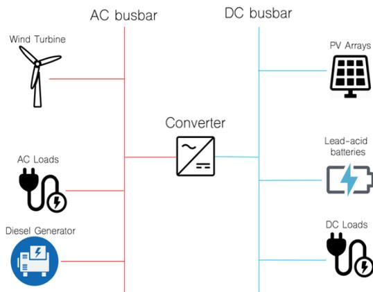
Fig. 1. Hybrid AC/DC Microgrid in isolated mode.
