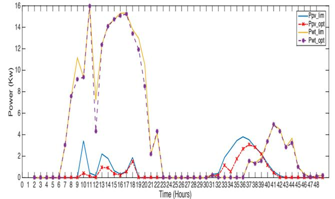
**Fig. 5.** Optimized power flow by HCS for off-grid mode.
