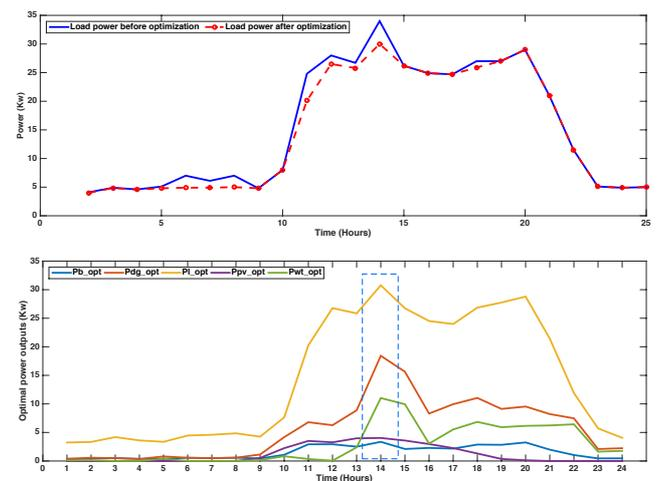
**Fig. 6.** HCS employing MILP optimization algorithm with Peak load case
