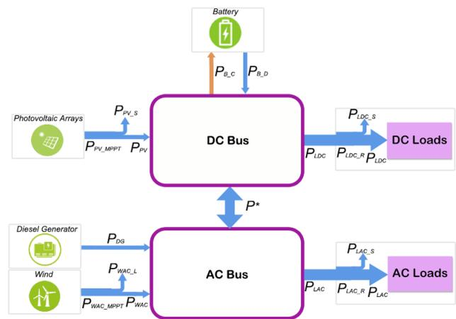
**Fig. 3.** Power flow in isolated mode.
