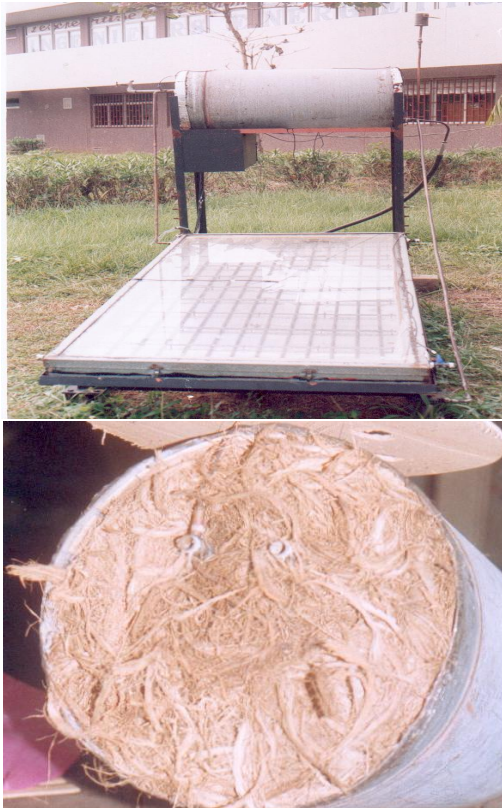
Fig. 2 Pictures showing one SWHS and the thermal insulation of one of them with the coconut fiber
