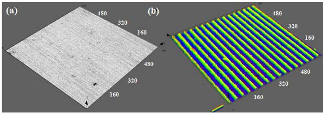
**Fig.4** Surface topography images of a) Plain sample, textured samples with a groove width of b) 30 μm
