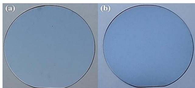
**Fig. 1** MC-Si wafer sample a) polished side b) un-polished side
