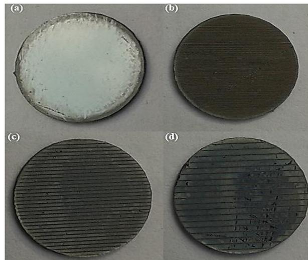
**Fig.2** Samples that are a) plain b) textured with a groove width of 30 $\mu$ m and pitch of 100 $\mu$ m c) textured with a pitch of 300  $\mu$ m and groove width of 30  $\mu$ m d) textured with a pitch of 500  $\mu$ m and groove width of 30  $\mu$ m
