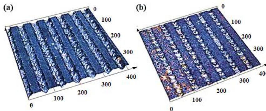
**Fig.5** Surface topography images of a) textured and etched sample with a groove width of 30 μm b) textured and etched sample with a groove width of 40 μm
