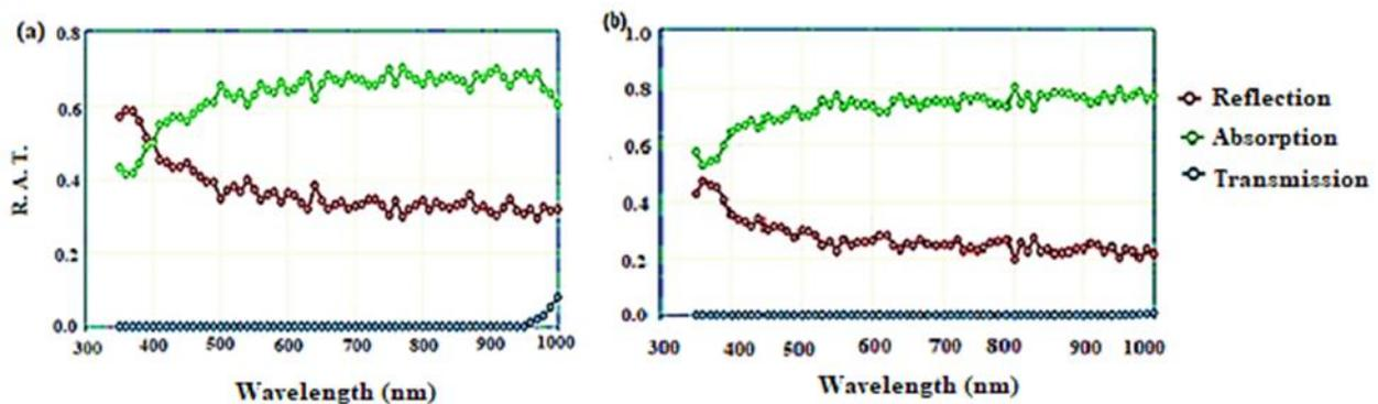
**Fig 3.** Percentage reflectance graphs for a) plain sample, (b) samples having a grooved front surface morphology with a groove size of 30 $\mu$ m
