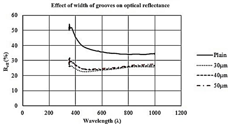
Fig.6. Effect of width of textured grooves on optical reflectance
