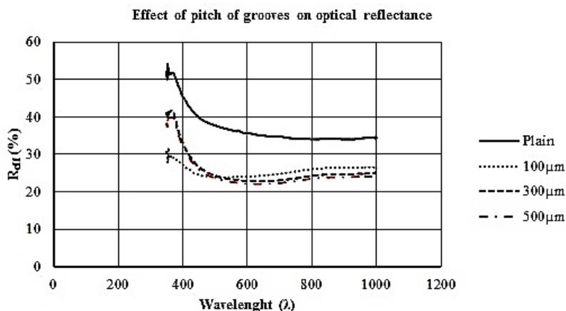
Fig.7 Effect of pitch of textured grooves on optical reflectance
