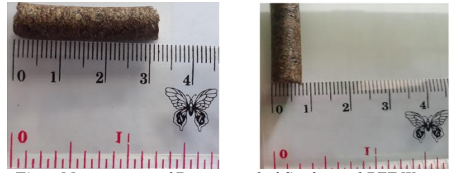
Fig. 2 Measurement of Dimensional of Garden and PET Waste into RDF Pellets
