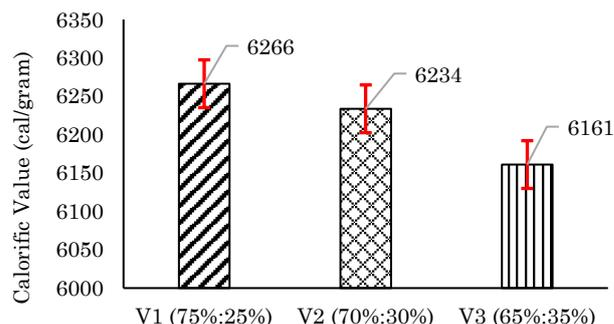
Fig. 6 Calorific value of coconut shell briquettes with cassava peel adhesive
