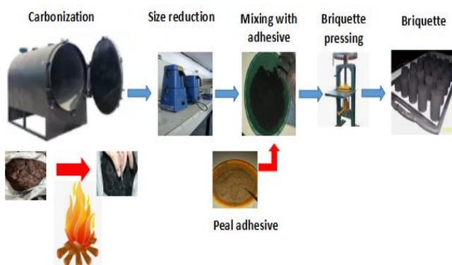
Fig. 1 Briquette preparation schematic diagram
