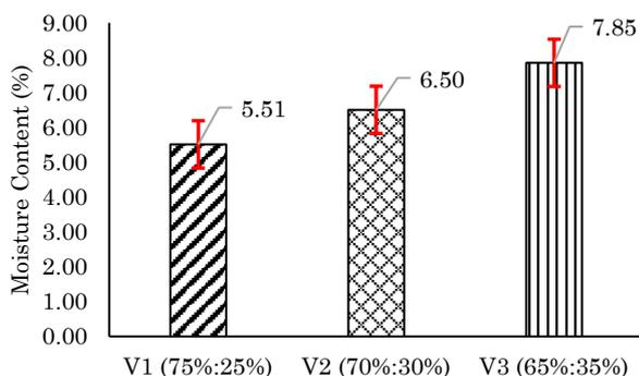
**Fig. 3** Moisture content of coconut shell briquettes with cassava peel adhesive
