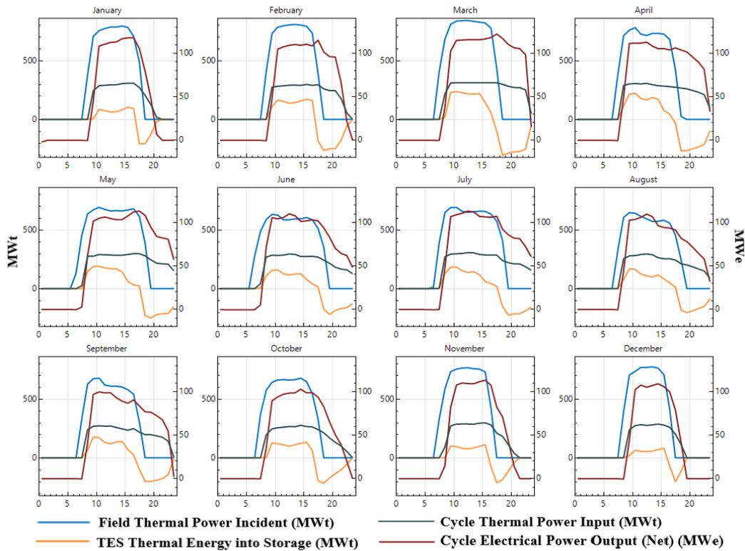
Fig. 3 Field incident solar thermal power, thermal power input for a power cycle and electrical output (Tamanrasset).
