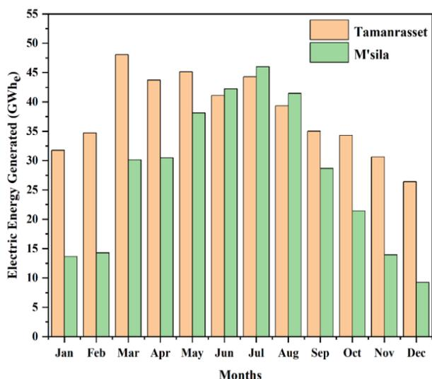
Fig. 5 Monthly energy generation for the proposed parabolic trough power plants in Algeria.
