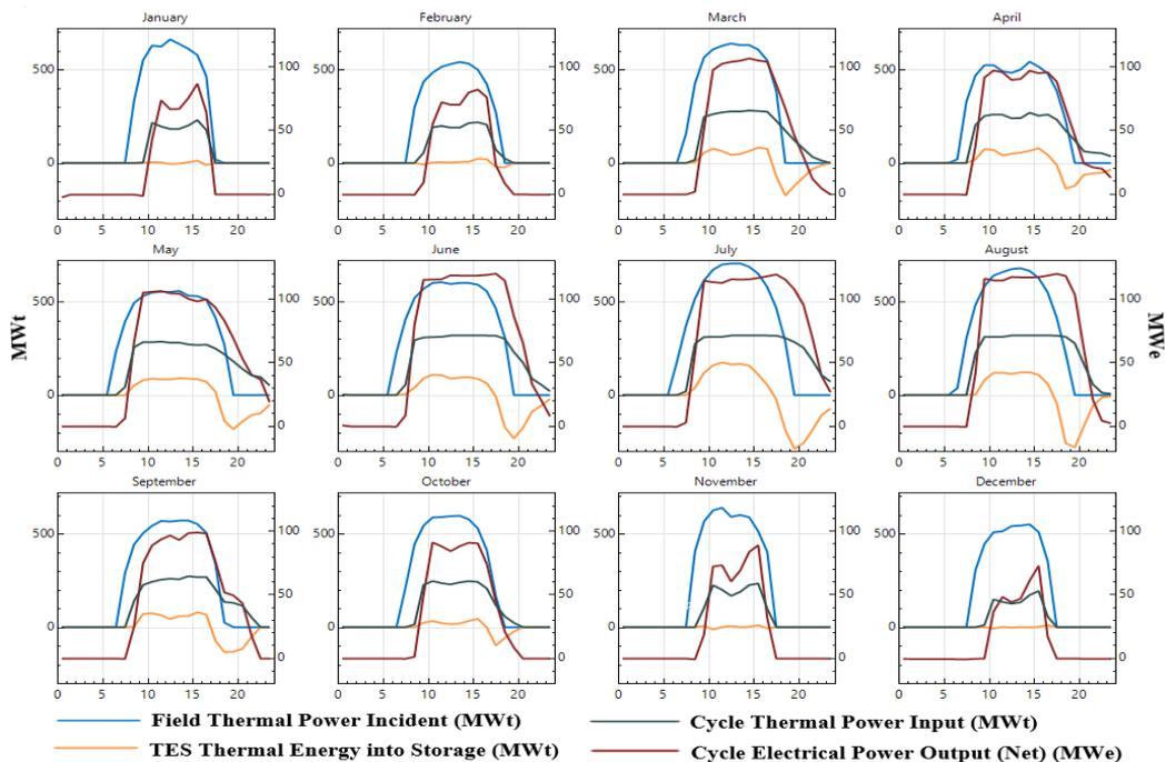
Fig. 4 Field incident solar thermal power, thermal power input for a power cycle and electrical output (M'Sila).
