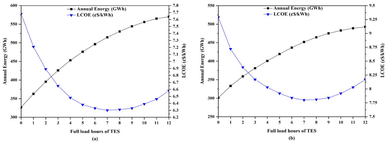
**Fig. 8** The variations of annual energy generation and LCOE with full load hours of TES of the proposed CSP plant in (a) Tamanrasset and (b) M'Sila.
