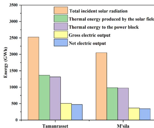
Fig. 6 Annual energy flow of the proposed parabolic trough power plants.
