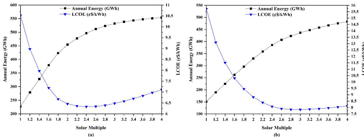
**Fig. 7** The variation of annual energy generation and LCOE with SM of the proposed CSP plant in: (a) Tamanrasset and (b) M'Sila.
