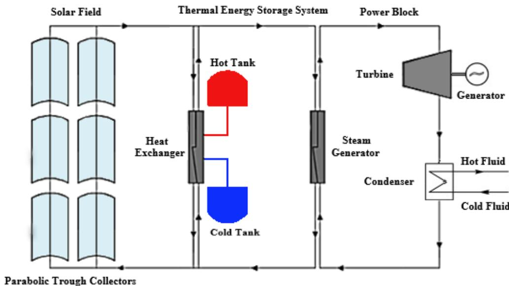
**Fig. 2** Schematic diagram of a parabolic trough CSP plant with TES system.
