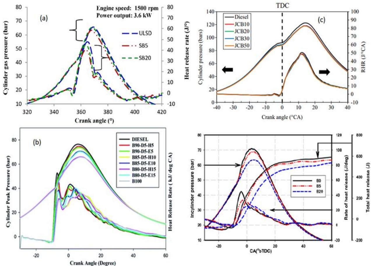
**Fig. 3.** The different between cylinder gas pressure and heat release rate with the crank angle of diesel fuel and different biodiesels (Ramalingam and Mahalakshmi, 2020; Seraç *et al.*, 2020; Silitonga *et al.*, 2017; Zarrinkolah and Hosseini, 2022)(a) soybean-based biodiesel (b) *Moringa oleifera* biodiesel (c) *Jatropa curcas* biodiesel (d) sunflower methyl ester biodiesel
