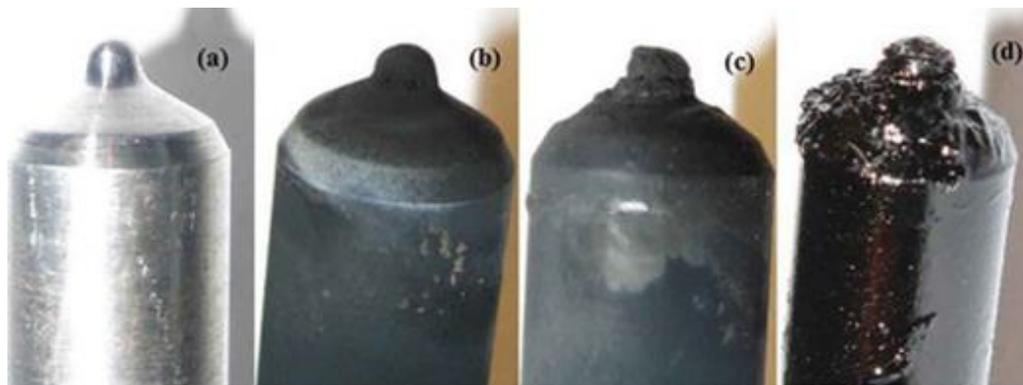
**Fig. 4.** The optical investigation for deposit formation level evaluation on injectors (a) new nozzle, (b) diesel fuel, (c) BD30, (d) BD100 (Birgel *et al.*, 2011)
