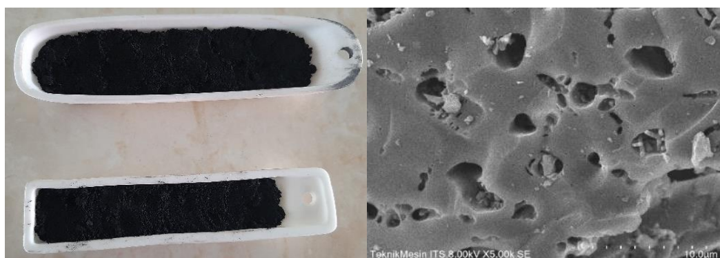
Fig 7. The optical image of AC700 powder (a), The SEM image of AC700 (b)
