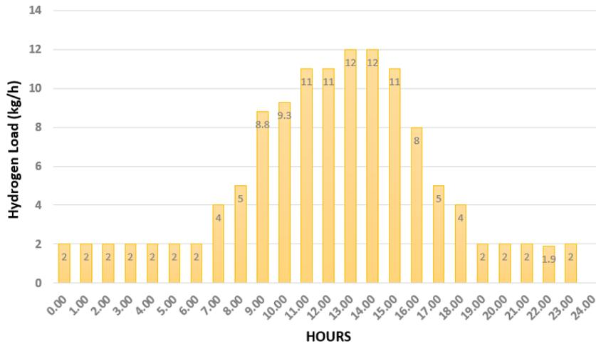
Fig. 7. Hourly H<sub>2</sub> load profile of typical refuelling day in the HRFS.
