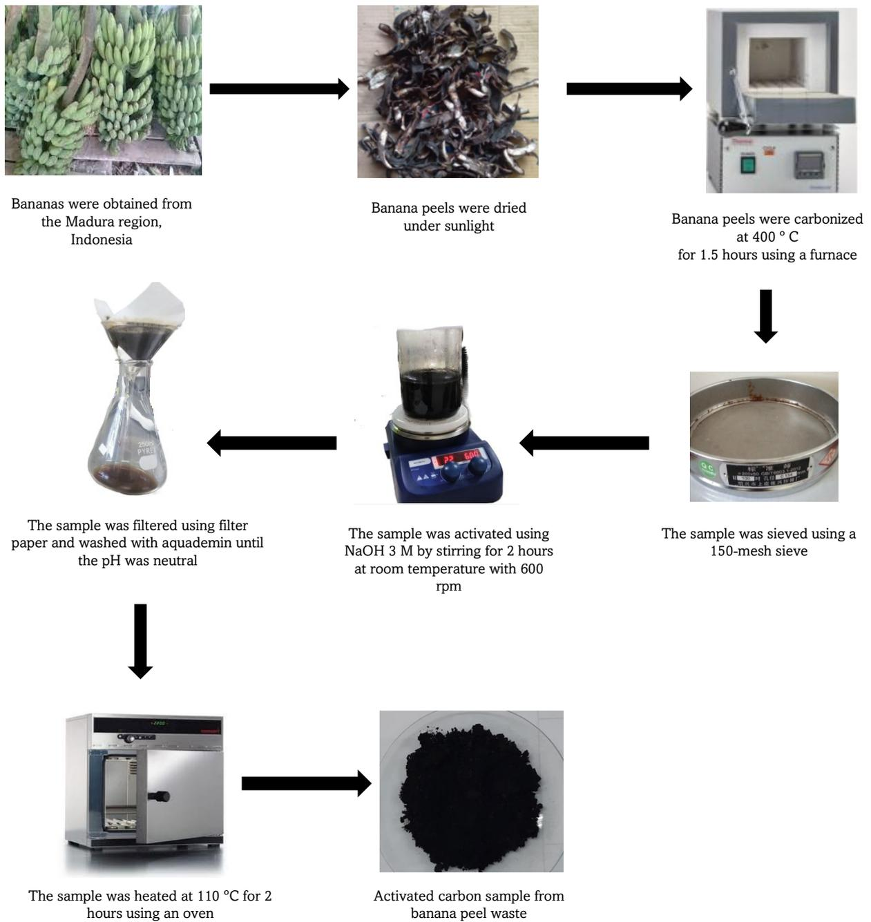
**Fig. 1** Preparation of activated carbon from banana peel waste
