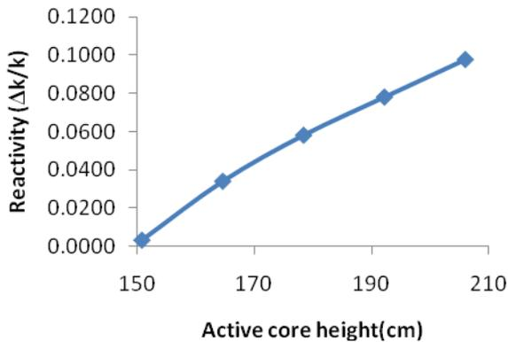
Figure 5. Reactor reactivity in each active core height
