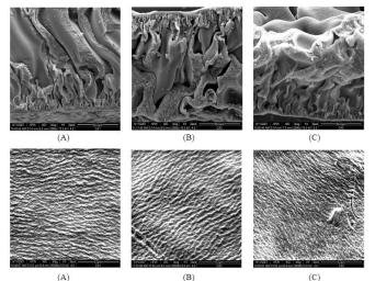
Fig. 1. SEM images (2000 x) of membrane surface morphology (below) and cross section morphology (above) made of 13 % CA in DMSO with different exposure time : (A) 1.75 sec (B) 2.33 sec; (C) 7.00 sec
