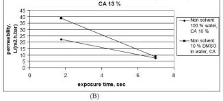
Fig. 4 The influence of the non solvent concentration to water permeability
