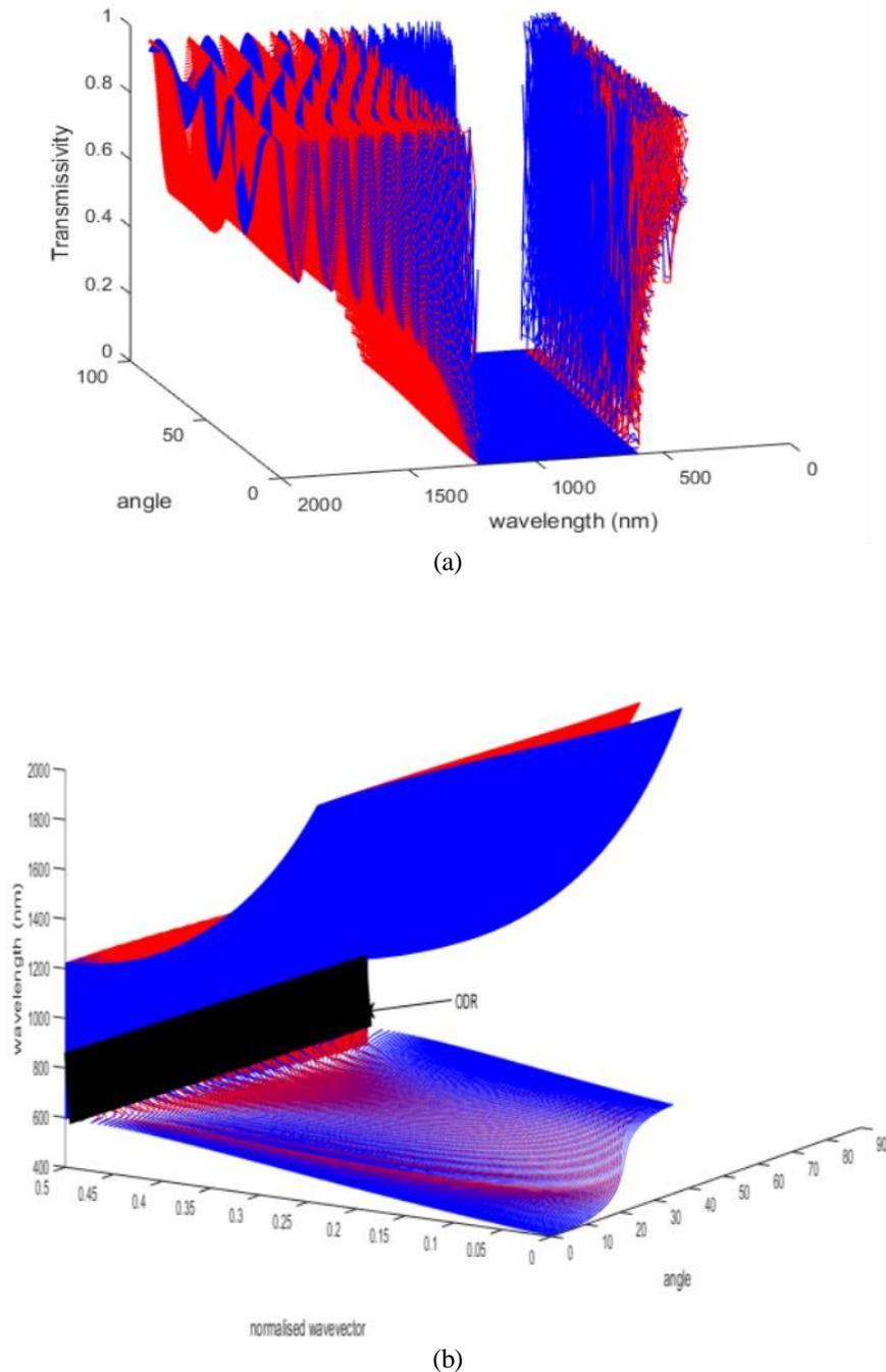
Figure 3: (a) Transmissivity variation with wavelength and angle of incidence (deg.) for TE modes (Red lines) and TM modes (Blue lines) in multilayered Cryolite-Ge (b) Dispersion relation with variation in angle of incidence (deg.) for TE modes (Red lines) and TM modes (Blue lines) in multilayered Cryolite-Ge.
