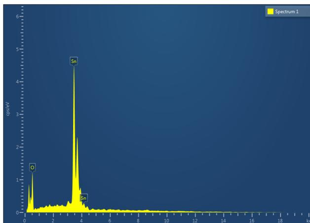
Figure 3. EDAX spectrum of SnO<sub>2</sub> nanoparticles
