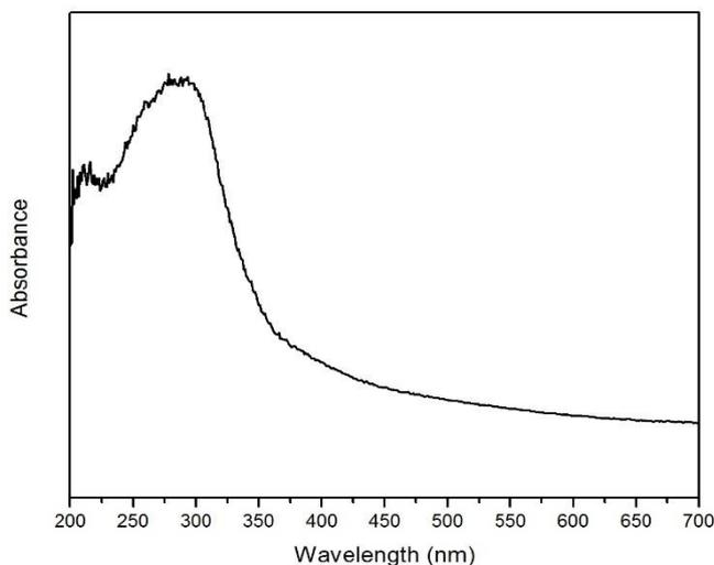
Figure 4. UV-Vis absorption pattern of SnO<sub>2</sub> nanoparticles
