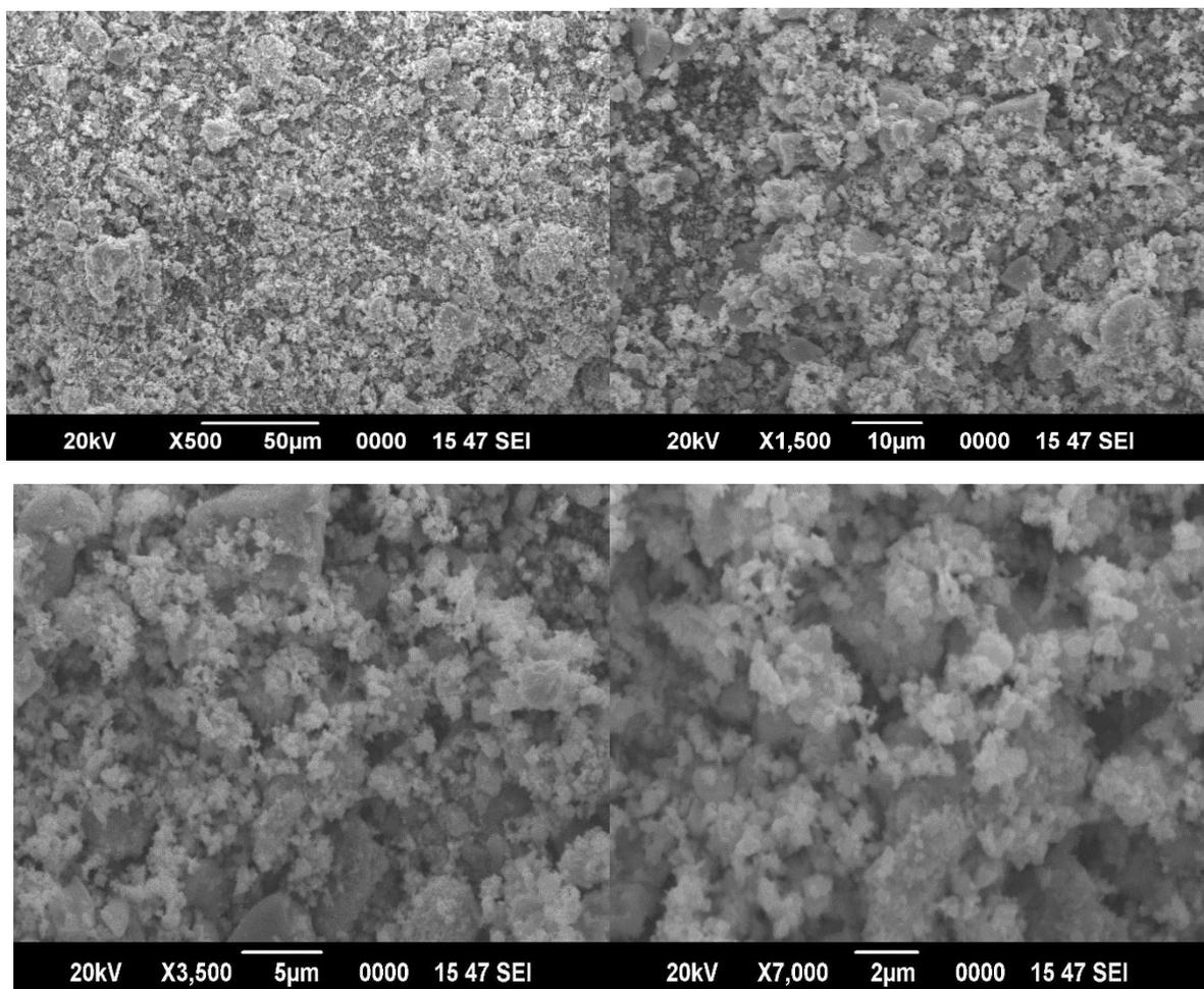
Figure 2. SEM images of SnO<sub>2</sub> nanoparticles
