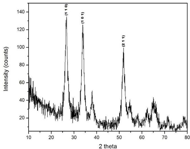
Figure 1. XRD pattern of SnO<sub>2</sub> nanoparticles
