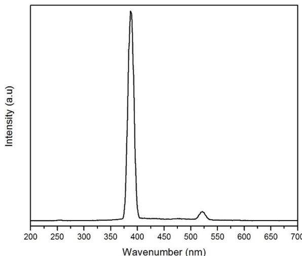
Figure 5. Photoluminescence pattern of SnO<sub>2</sub> nanoparticles
