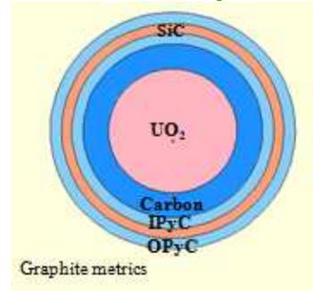
Figure 4. MCNP model of coated fuel particle (TRISO)
