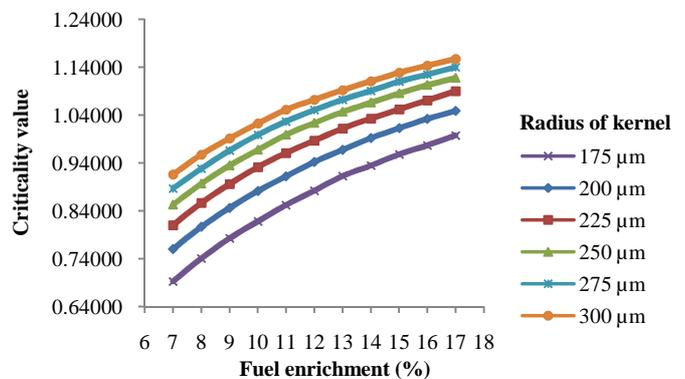
Figure 8. Graph criticality value of reactor with fully out control rod
