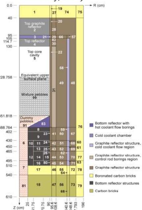
Figure 2. HTR-10 reactor vertical cross-section (W. Terry, 2006)
