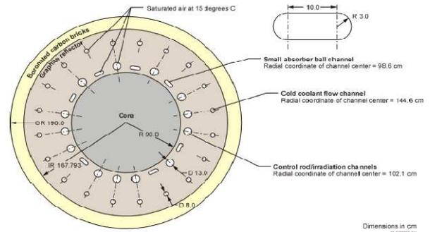
Figure 1. HTR-10 reactor horizontal cross-section (W. Terry, 2006)
