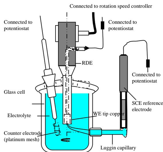
Figure 1 Diagram of three-electrode cell for electrochemical investigation
