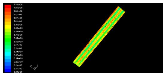
Fig. 8: Contour flow patterns in sub channel with fuel element rectangular arrangement using nanofluid Al<sub>2</sub>O<sub>3</sub>-water (3%)
