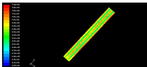
Fig. 7: Contour flow patterns in sub channel with fuel element rectangular arrangement using nanofluid Al<sub>2</sub>O<sub>3</sub>-water (2%)
