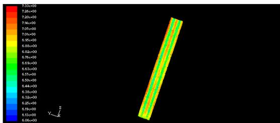
Fig. 5: Contours of the flow pattern in sub channel with fuel element rectangular arrangement using light water (H<sub>2</sub>O)
