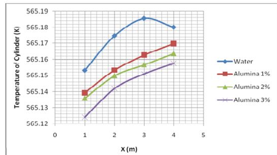
Fig.11: Distribution of temperature in the cylinder wall heater in the sub channel rectangular arrangement
