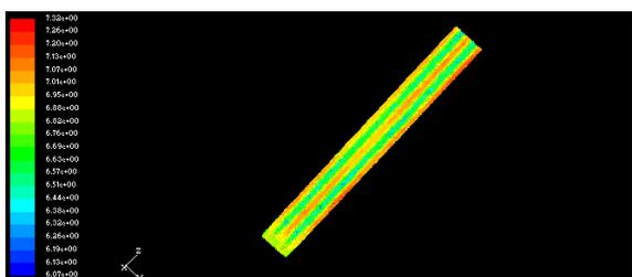
Fig. 6: Contour flow patterns in sub channel with fuel element rectangular arrangement using nanofluid Al<sub>2</sub>O<sub>3</sub>-water (1%)
