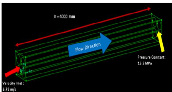
Fig. 3: Modeling sub channel rectangular arrangement in PWR reactor core
