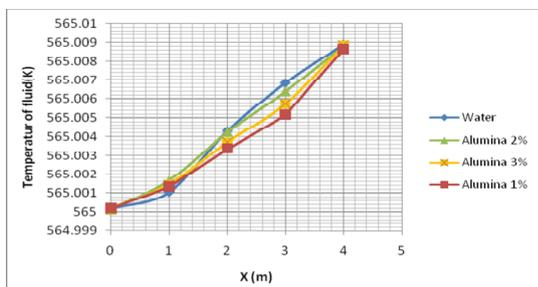
Fig. 10: Distribution of the temperature of the fluid that occurs in sub channel rectangular arrangement
