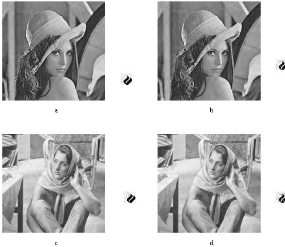
Fig. 9 (a) Lena (rate=4bpp, PSNR 39.661 dB, extracted secret image SIM = 0.9812). (b) Lena (rate=2bpp, PSNR 37.380 dB, extracted secret image SIM =0.8778). (c) Barbara (rate=4 bpp, PSNR 39.97 dB, extracted secret image SIM =0.9905). (d) Barbara (rate=2bpp, PSNR 38.4908 dB, extracted secret image SIM =0.8928)
