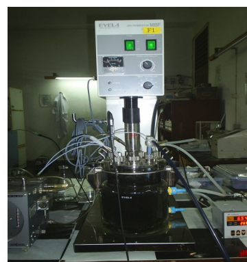
Fig. 1. Two-litre biodigester used for POME fermentation
