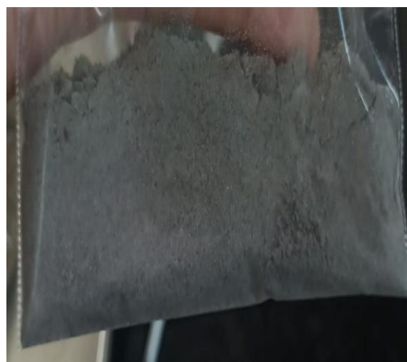
Figure 3. Shape And Color of Silica from Snake Fruit Ash
