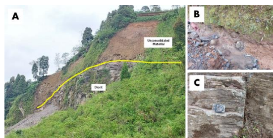
Figure 7. A) Depicts the Stratigraphic Position of the Unconsolidated Unit Overlying the Diorite Unit. (B) Close-up Image of the Unconsolidated Unit Containing Diorite Fragments. (C) Close-up Image of the Fresh Diorite Unit Exhibiting a 'Sheeting-Joint' Structure
