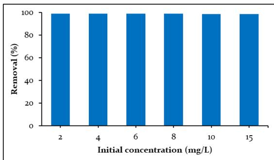
Figure 5. Effect of Initial Concentration on Zn (II) Ions Adsorption (pH 6, Dose 2 g/l, Contact Time 120 Minutes)
