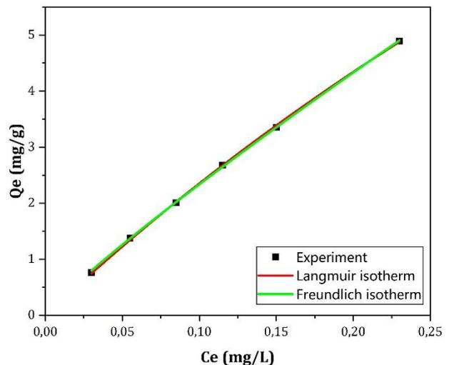
Figure 6. Adsorption isotherm of Zn (II) ions
