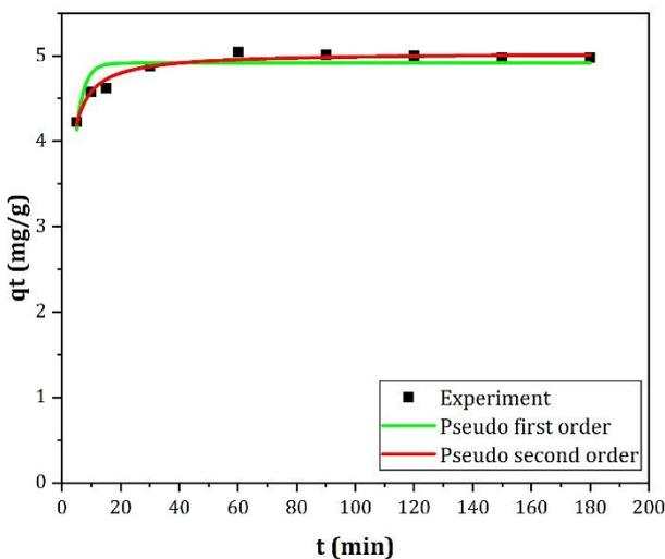
Figure 7. Kinetics of Zn (II) Adsorption
