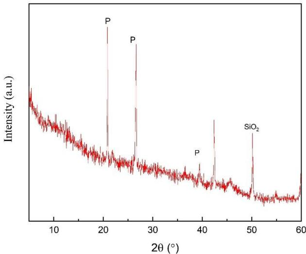
Figure 1. Zeolite XRD Result
