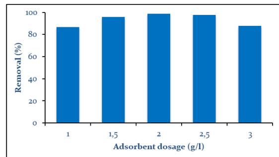
Figure 3. Effect of Adsorbent Dosage on Zn (II) Adsorption (pH, Contact Time 60 Minutes, Initial Concentration 10 mg/g)
