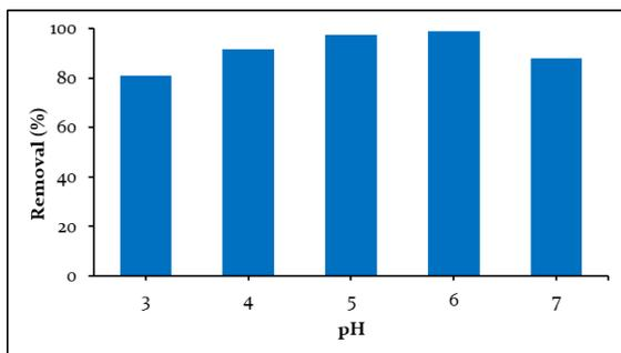
Figure 2. Effect of pH on Zn (II) Adsorption (dose 2 g/l, Contact Time 60 Minutes, Initial Concentration 10 mg/g)
