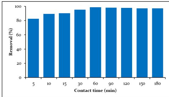
Figure 4. Effect of Contact Time on Zn (II) Adsorption (pH 6, Dose 2 g/l, Initial Concentration 10 mg/l)
