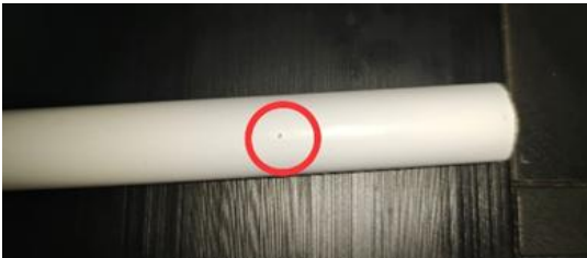
Gambar 4. Cacat Noda Gram
