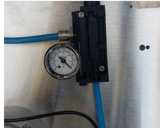
Figure 25. Vacuum Gauge Setup of Cartoner Machine
