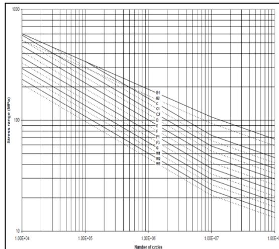
Figure 10. S-N Curve In Air [22]
