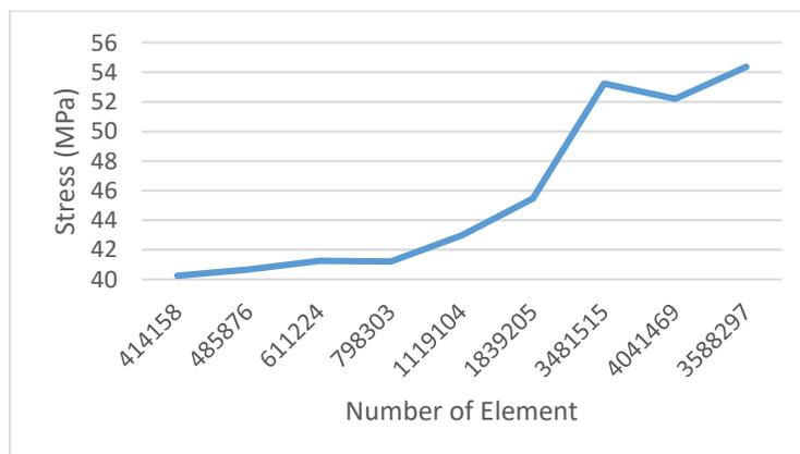
Figure 9. Stress Compare to the Element Size
