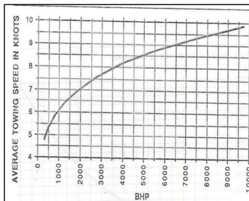
Figure 5. Towing Speed Vs Brake Horsepower Graph [16]
