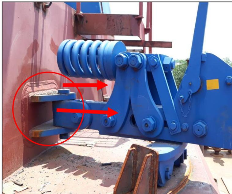
Figure 3. Model of Towing Hook Construction In Red Circle
