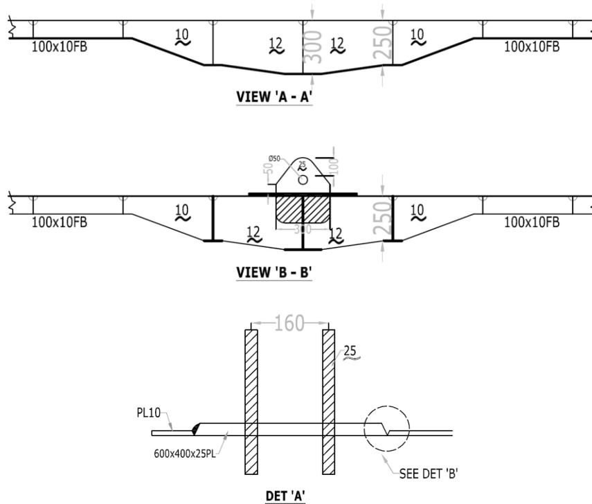
Figure 4. Detail of Towing Hook Construction
