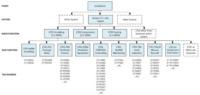
Figure 8. An example of an asset hierarchy based on Norsok Z-008 [8]
