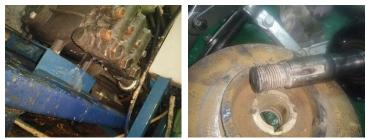
Figure 7. Malfunction of the High Pressure Reverse Osmosis Unit pump (Left), Damage to "spi" housing and seawater cooling pump impeller axle (Right)
