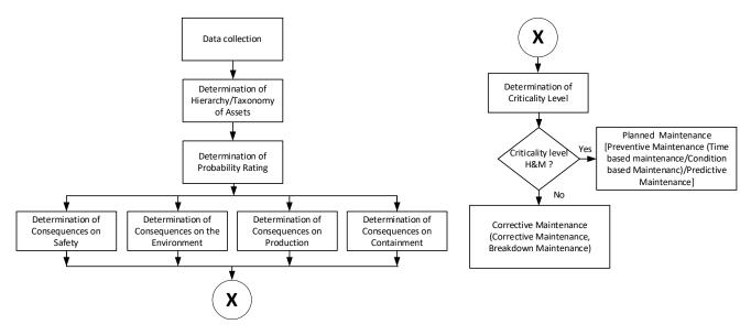
Figure 1. Critical analysis methodology flowchart
