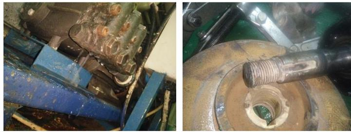
Figure 7. Malfunction of the High Pressure Reverse Osmosis Unit pump (Left), Damage to “ spi” housing and seawater cooling pump impeller axle (Right)
