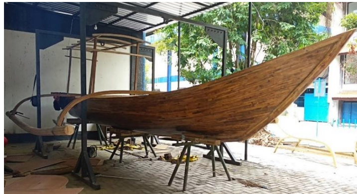
Figure 2. The 2 nd prototype of a coastal fishing boat made of laminated bamboo slats
