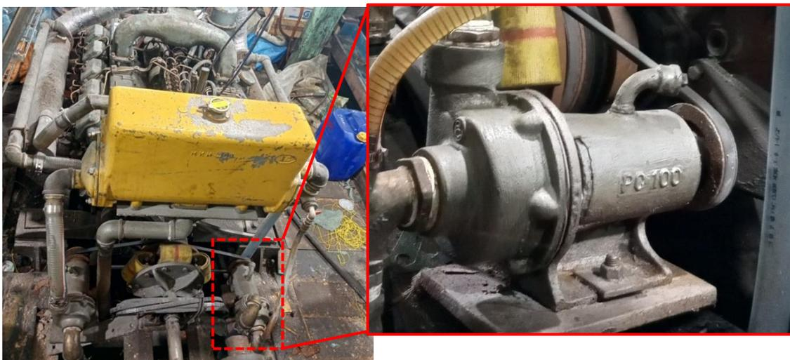
Figure 3. Centrifugal pump on fishing vessel main engine
