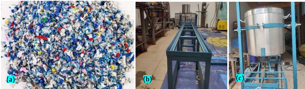
Figure 1. (a) Shredded plastic waste, (b) Jig-set for Recycled Plastic Waste Board Manufacture, (c) stainless steel heating pot.
