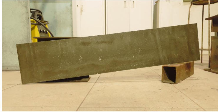
Figure 3. The Recycled Plastic Waste Board manufactured using heating pot and molds.
