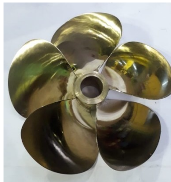
Figure 1. High-speed vessel (OPV 98 M) propeller model
