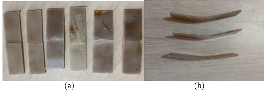
Figure 7. The shape of the test specimen after testing: (a) broken test specimen, (b) bent test specimen
