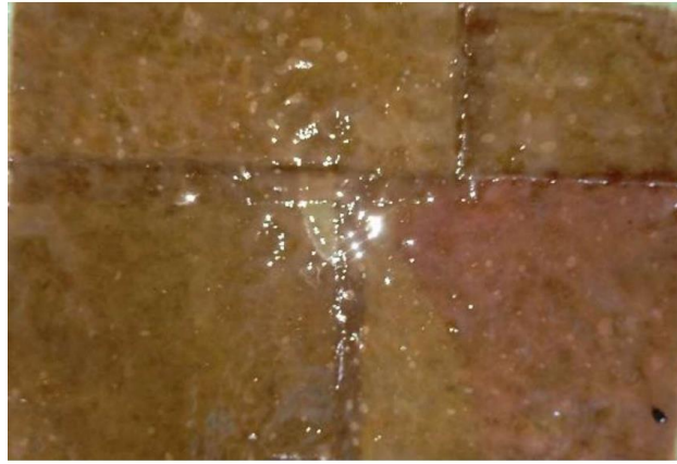
Figure 4. Example of resin-coated cardboard test specimen
