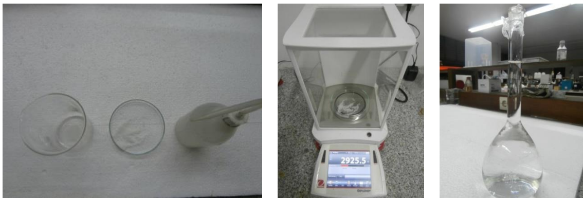
Figure 4. Preparation of electrolyte liquid NaCl 0.1 M
