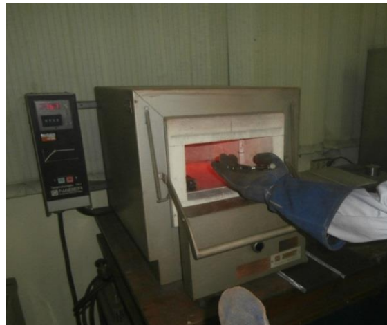
Figure 1. Simulation of burnt ship plates in Furnace
