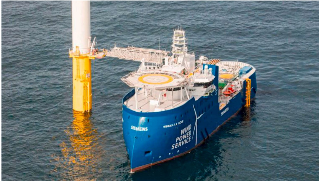
Figure 1. Illustration of a CSOV vessel with Gangway in operation [3]
